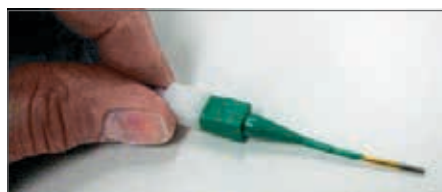
Plastic tool with contact in proper position.
