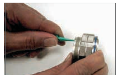
Plastic tool with contact in proper position.
